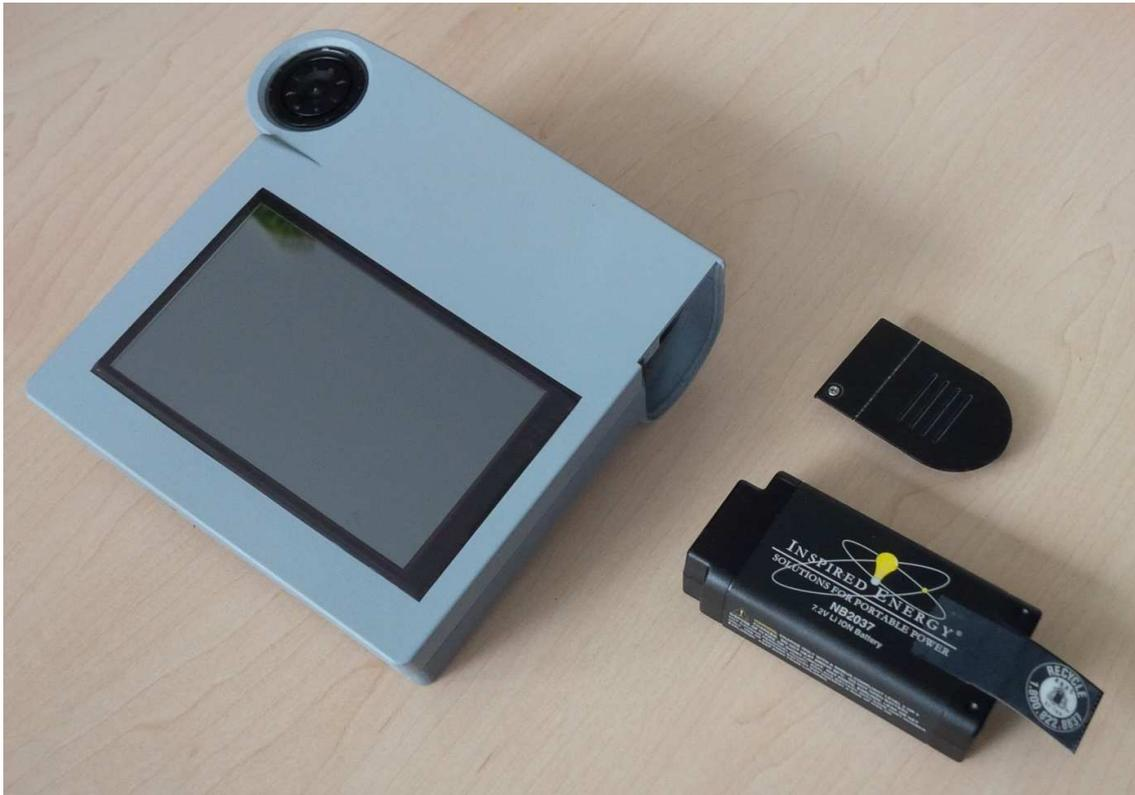
Figure 1: MobilePass-Device with exchangeable Li-Ion - Accumulator.
