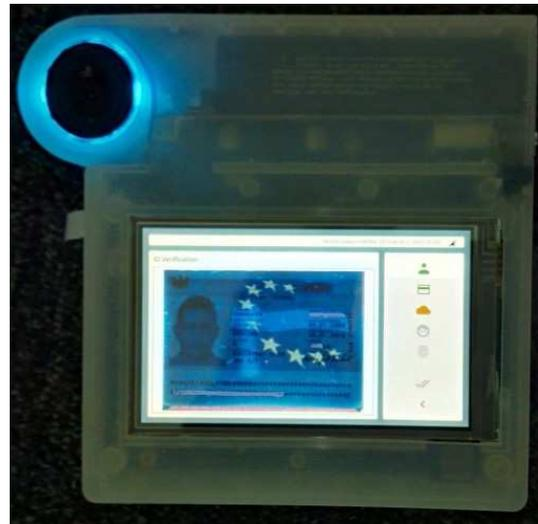
Figure 3: Device display of IR and UV Image scans - © MobilePass Consortium
